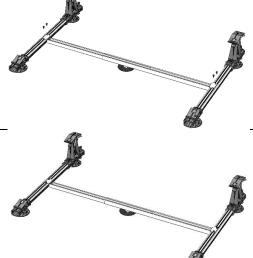
6. Fix the anchorbar to the FlatFix Fusion profiles with 4x screw 6,0x25mm. Art. Nr. 100-3010.
