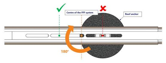
Make sure the front side of the anchor bar is always touching the FlatFix Fusion profile.
