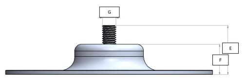
The dimensions of a roof anchor should always be within range defined in the table below. The above figure shows the positions of these dimensions.
