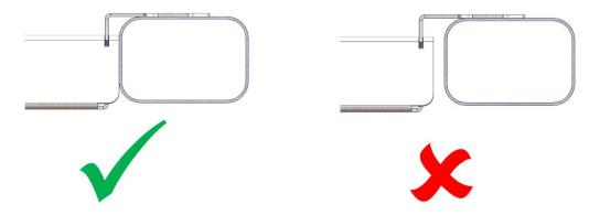
Mount the anchor bar to the FFF profiles.
