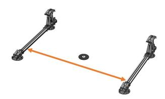
Make sure the system is aligned correctly for the right panel size. Mark the outlines of the panel field on the roof with chalk or a marker.
