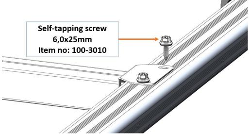
Fasten the anchor bar to the roof anchor.
