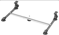
5. Fix the anchorbar with a M10 washer and nut. Min. torque is 10Nm.
