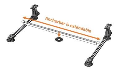
Extend the anchor bar to fit between the two rails.
