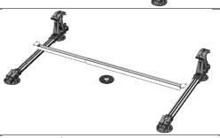
4. Place the extendable anchorbar, make sure the anchorbar is extended in full and touches the FlatFix Fusion frame completely, leaving no gaps.
