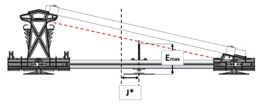
The height of the anchor base should not exceed 21,5 mm. If it does, the anchor will lift the Anchor Bar and the FFF system from the roof and make the system more vulnerable for wind sheers resulting in damage to the panels and system.
